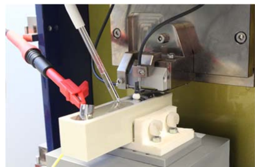
Tribokorrosionsaufbau im Mikrolast-Tribometer Electrochemical-Cell-Unit at the Low-Load Tribometer
