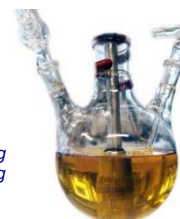
Sensorsystem (im Ölbad) zur Ölzustandsüberwachung Sensor system (in oil bath) for Oil-Condition-Monitoring
