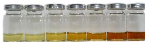
Öl in verschiedenen Alterungsphasen (von links nach rechts) / Infrared Oil in different conditions during artificial alteration (from right to left: increasing degree of deterioration)
